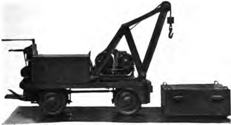
FIG. 5.—4,000-LB. CARRYING CRANE AND DUAL BATTERY EQUIPMENT
